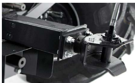
Rear tow hook approved for trailers up to 6,000 kg (optional hydraulic or pneumatic braking system for towing up to 14,000 kg).
