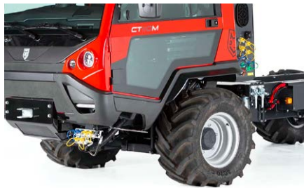
Different hydraulic versions available with lever or joystick controls for 3, 4, or 5 elements, quick couplings in front of and/or behind the cab.
