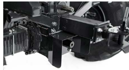
Power take-offs with independent hydraulic clutch, upper output at 540/1000 rpm and/or lower output at 540 rpm on rear axle with electro-hydraulic control.
